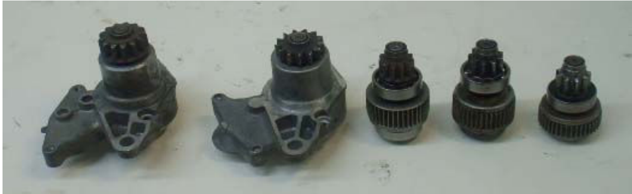
Nippondenso drives which can be fully rebuilt including removing ball bearings and replace the inside rollers and springs.
