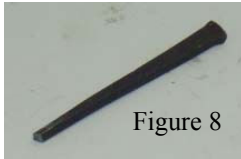
K108-0700-9 Tool to open the snap ring
