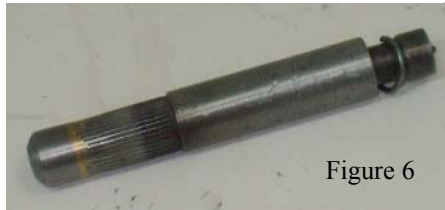
K108-0700-07 Tool to insert the reusable snap ring.
