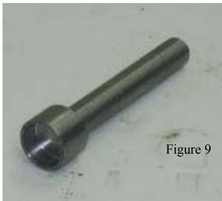
K108-0700-10 Tool to release the snap ring from the snap ring retainer
