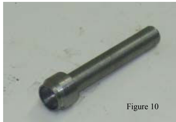
K108-0700-11 Tool to insert the snap ring in the snap ring retainer
